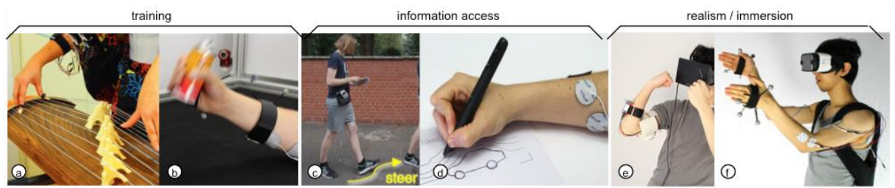
Figure 1: Examples of interfaces, which actuate the users by means of electrical muscle stimulation.
