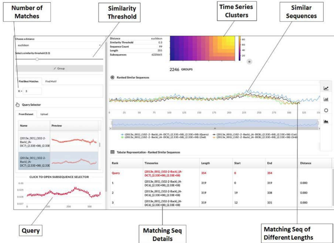
Figure 1. Snapshot of the BrainEx interface showcasing exploration and retrieval of similar sequences of data. This can be valuable in the early stages of development of neuroadaptive technology. From left to right we display a scenario where the analyst chose a specific query sequence from a dataset and is retrieving the three most similar matches (displayed on center right panel). The similarity exploration uses Dynamic Time Warping, which enables the retrieval of similar sequences of different lengths and with temporal misalignments. The top right panel shows statistics about the natural distribution of time series in clusters for specific lengths, contributing to better understanding of the data. Left lower panel displays the ability to select subsequences of time series and use them as queries, while right lower panel gives information about the results including patient, channel, start, end and length of the matching sequence. The analyst can display/hide the matching sequences as needed for better visualization and interpretation.
