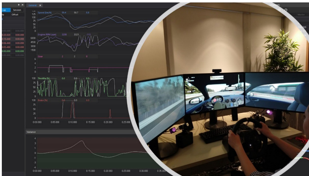
Figure 1. Driving Simulator, Eye Tracker, Camera Setup, overlaid upon Telemetry collected in parallel with driving Simulation.
